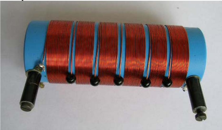
Completed coil with antenna & Diode Taps:
