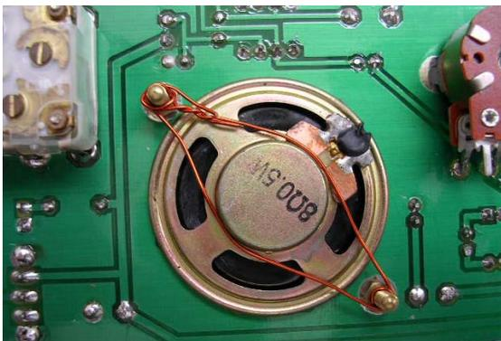
**Picture shows how a speaker may be fixed on the PCb by way of using support of two brass bolts.**
