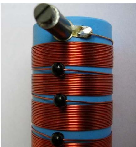
**Start winding coil as illustrated in picture at left.**
