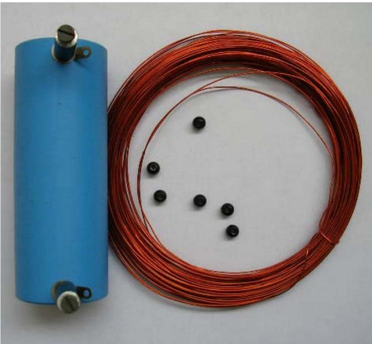
Coil kit consists of an enameled copper wire, few glass beads and a PVC pipe with aluminum stands, lugs and bolts.
